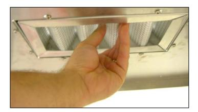
1. Clean the filter in warm soapy water, and allow to dry overnight. Replace the filter by putting it into the slot, and pushing upward. (As shown below) Make sure the filter frame is flush with the roof of the machine. (As shown above)
