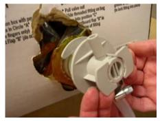
3. Connector shown with shell correctly engaged and plunger forward in lock position. Oil flow commences.
