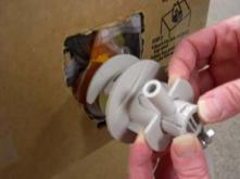
2. With the hose connector in place, place fingers behind flange on connector and press plunger forward to lock.
