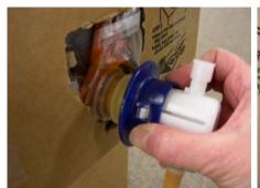
3. Connector shown with shell correctly engaged and collar forward in lock position. Oil flow commences. *Do not slide crosspiece forward.*
