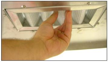
3. Clean the filter in warm soapy water, and allow to dry overnight. Replace the filter by putting it into the slot, and pushing upward. (As shown below) Make sure the filter frame is flush with the roof of the machine. (As shown above)
