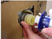
1. With the blue collar on the hose connector retracted toward crosspiece, slide hose connector shell onto bag nozzle.
