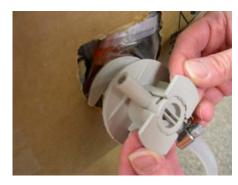
3. Connector shown with shell correctly engaged and plunger forward in lock position. Since the White Insert Bag Nozzle is not designed to work with the insert pressed forward, this configuration may or may not work. If it does not, remove the gray hose connector and order the blue hose connector from Gold Medal.
