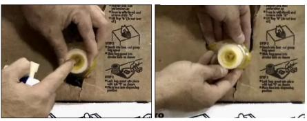
**NOTE:** If the oil does not flow after engaging plunger on gray hose connector, or if the crosspiece is inadvertently pushed forward when using the blue hose connector with the white insert nozzle, the nozzle center slider insert will be left pushed back into the bag, as shown above left.
