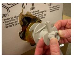
2. With the hose connector in place, place fingers behind flange on connector and press plunger forward to lock.
