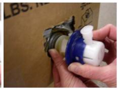
2. Holding the bag connector, slide the blue collar forward to lock the hose connector onto the bag nozzle.
