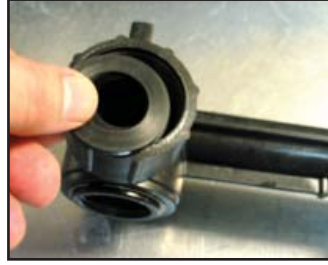
F. Ensure gaskets are installed in both connections of bypass assy
