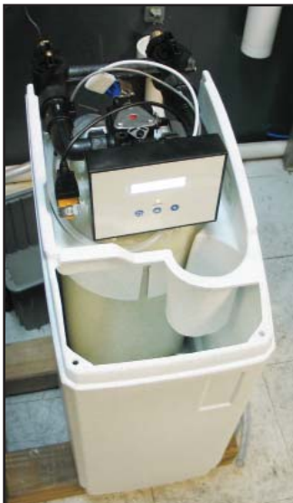
A. Softener with covers removed
