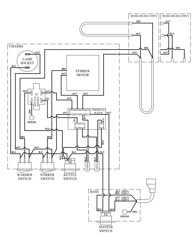
TP-16 WIRING DIAGRAM (120V)
