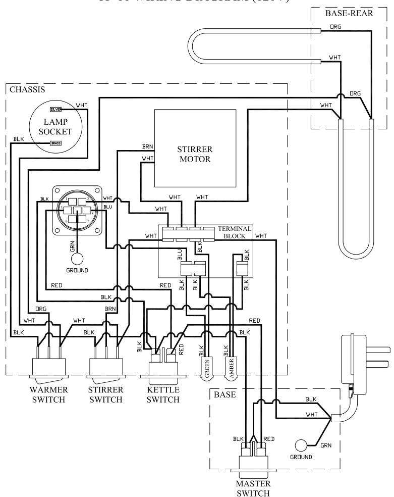
TP-16 WIRING DIAGRAM (230V)
